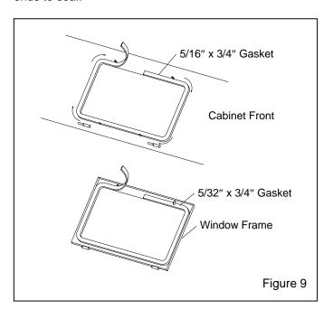
**7.4.5** Using 5/32" thick strip gasket, repeat the process on the window frame.
