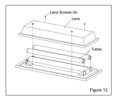
**7.6.3.3** Remove the four lens screws and remove the lens.
