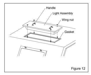
**7.6.2.3** Lay a section of strip gasket next to the opening, and cut to length, allowing 3/4" overlap on each end. Peel a short section of adhesive backing and adhere the strip gasket to the top edge of the light opening, as shown in Figure 12. Press the gasket tightly to bond. Repeat the process for each side, compressing the ends to seal.
