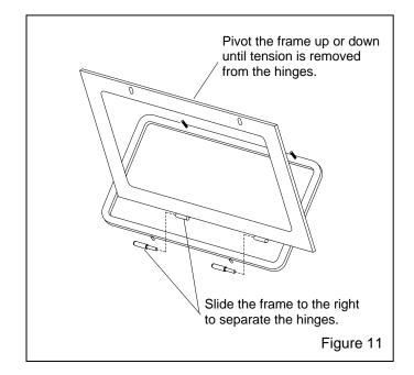
**7.5.4** Slide the frame to the right, to remove. The hinges separate as shown in Figure 11.
