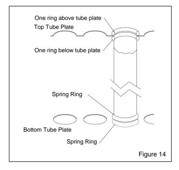
**7.7.2** The tubular filter is held firmly by spring rings above and below the perimeter of the hole in the top and bottom tube plate. The filters fit tight to prevent dust leakage. Force may be required by the installer. Check for proper seating at both ends, and remove any twist in the tube before proceeding to the next filter.
