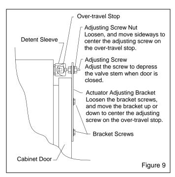
**5.6.5** Test the operation with the doors open and then again closed. Point the nozzle away from the door during the tests, and only open the door enough to disengage the interlock switch. The interlocks should stop the blasting when the doors are opened, and permit blasting when the doors are closed. NOTE: Negative pressure inside the cabinet may cause the doors to flex inward. Tests should be performed with the exhauster running.
