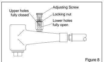
**5.3.3** If pulsation occurs in the media hose, either media is damp and caked, or not enough air is entering the media stream. While blasting, loosen the locking nut and slowly
