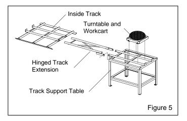
**3.4.2** Place the inside track in the cabinet over the existing grate as shown in Figure 6.
