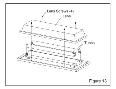
**7.6.3.3** Remove the four lens screws and remove the lens.
