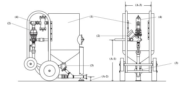
**Nominal** Shipping **Dimensions** (including skid) Unit Height (floor to highest point):  $53^{1}/2$ " 59" Width (outside hub to hub): 29" 35" 51" 52" Length (hose cplg. to handle): Machine diameter: 24" Net weight: 514 lb Shipping Volume: 62.1 cu ft Shipping Weight: 588 lb
