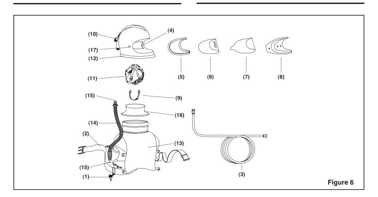
is notched. Continue sliding the cape around the bottom of the helmet until the entire cape is completely into the groove. NOTE: Spraying a non-toxic silicone-base lubricant into the groove will reduce friction and ease assembly.
