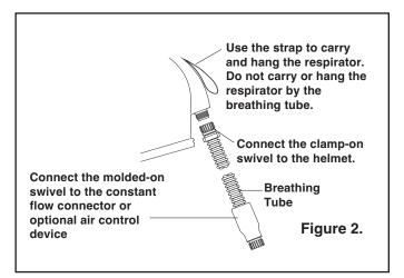
**3.4.2** Attach the molded-on swivel connector to the Constant-Flow Connector, or alternate air control device.
