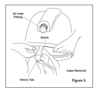
**9.4.3** Slide the ends of the cape to the notch. Continue sliding one end of the cape out of the groove until the entire cape is detached from the helmet.
