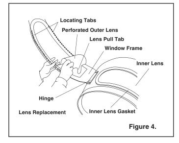
**9.2.1** Up to five outer lenses can be installed at one time. For maximum visibility, install only enough lenses to last during a work period.
