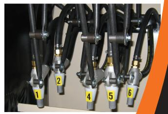
**Six or Four Blast Guns** mounted on separately adjustable holders enable operators to control blast coverage.
