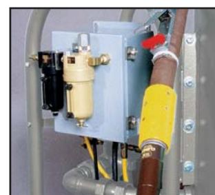
The Millennium pneumatic remote control valve combines inlet and outlet functions.
