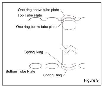
**7.4.2** The tubular filter is held firmly by spring rings above and below the perimeter of the hole in the top and bottom tube plate. The filters fit tight to prevent dust leakage. Force may be required by the installer. Check for proper seating at both ends, and remove any twist in the tube before proceeding to the next filter.
