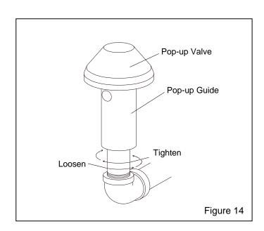
**6.8.5** Slide the new pop-up valve over the guide, and then screw the valve guide (with the pop-up valve on it) into position inside the machine. Tighten the guide snug, but not wrench-tight. Over-tightening the guide will make it difficult to remove the next time the pop-up valve needs replacement.
