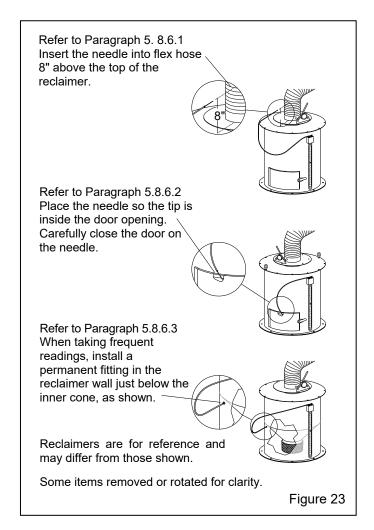
**5.8.6.2 Taking readings at the reclaimer door:** Open the reclaimer fill door, remove the needle protector, and place the needle so the tip is inside the door opening. Carefully close the door on the needle. The side of the needle will embed into the rubber, creating an airtight seal.
