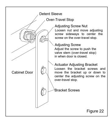
**5.7.5** Test the operation with the door open and then closed. Negative pressure inside the cabinet may cause the door to flex inward. Tests should be performed with the exhauster running. Point the nozzle away from the door during the tests and open the door only enough to disengage the interlock switch. The interlocks should stop the blasting when the door is open and permit blasting when the door is closed.
