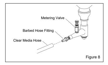
**2.6.1** Refer to Figure 8 and attach the clear media hose from under the cabinet hopper to the metering valve at the bottom of the reclaimer hopper by sliding the hose onto the barded fitting on the metering valve.
