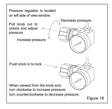
**5.1.2** To adjust pressure, unlock the knob by pulling it out, as shown in Figure 18, and turn it clockwise to increase pressure or counterclockwise to decrease pressure. Pressure may drop slightly from closed-line pressure when blasting starts. Once operating pressure is set, push the knob in to lock it to maintain the setting.
