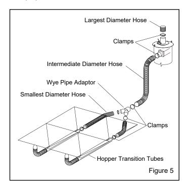
**2.2.3** The largest diameter hose attaches between the reclaimer outlet and dust collector inlet.
