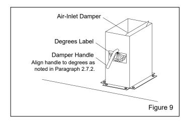
**2.7.2** The label on the damper shows the settings in degrees. The initial setting should align the handle as follows:
