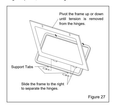
**7.6.5** Replace the frame in reverse order. Align the top bolt holes with the bolts; slide the frame as necessary.
