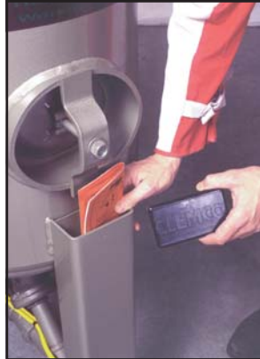
Weather-tight storage bin in front leg to keep manuals.
