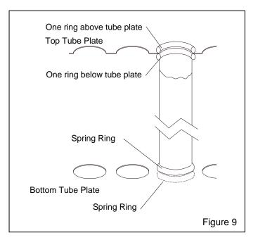
**7.6.2** The tubular filter is held firmly by spring rings above and below the perimeter of the hole in the top and bottom tube plate. The filters fit tight to prevent dust leakage. Force may be required by the installer. Check for proper seating at both ends, and remove any twist in the tube before proceeding to the next filter.
