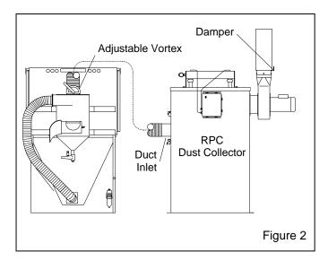
**1.5.3 Reverse Pulse Dust Collector:** A pull-through reverse-pulse dust collector is the most efficient dust collector option. Cartridge filters are automatically cleaned by a periodic pulse of compressed air. This type of dust collector used with the optional HEPA filter must be used in applications in which toxic dust is generated. See separate manual for operation of reverse-pulse dust collectors.
