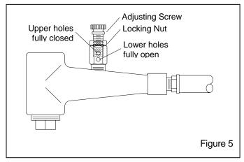
**5.3.3** If pulsation occurs in the media hose, either media is damp and caked, or not enough air is entering the media stream. While blasting, loosen the locking nut and slowly turn the adjusting screw out (counterclockwise when
